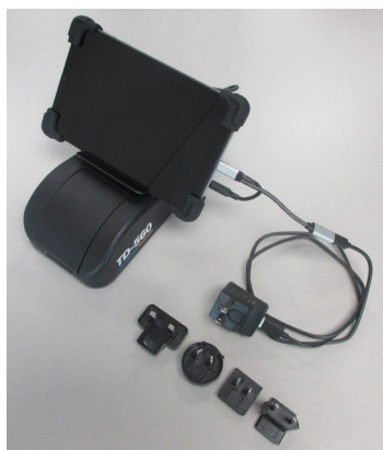
Front and back views of the analyzer, showing sample well, touch-screen tablet, cables and power adapters.
